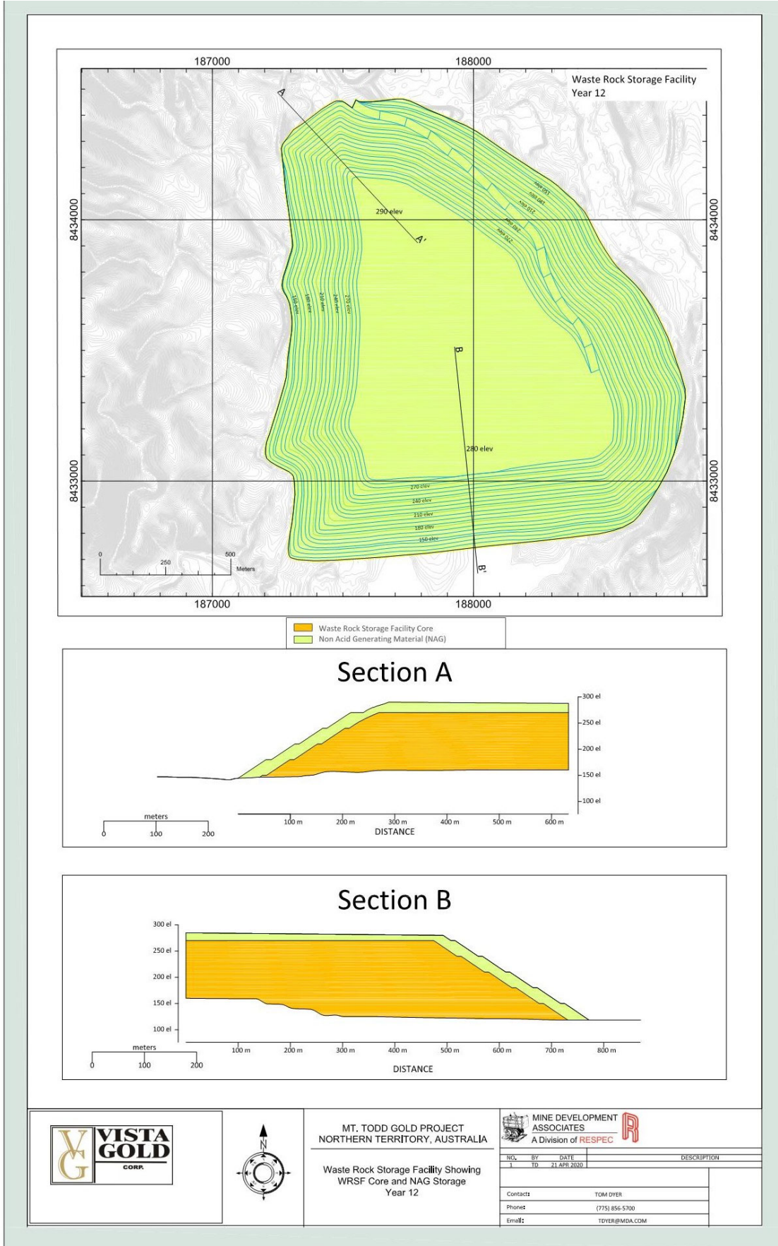
Figure 4-13 Waste Rock Dump Year 12- At Completion
