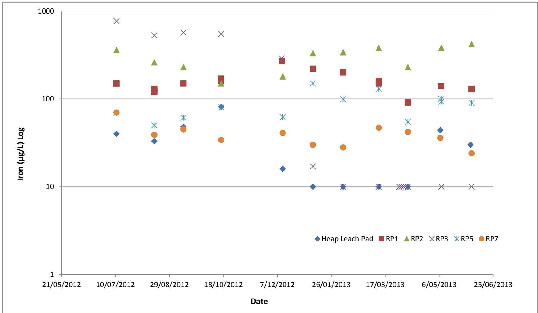
Figure 52 - 0.45 µm filtered Iron concentrations in primary retention ponds
