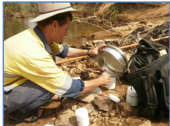
Figure 9. Transfer of sieved sample to jars for preservation and transport back to lab.
